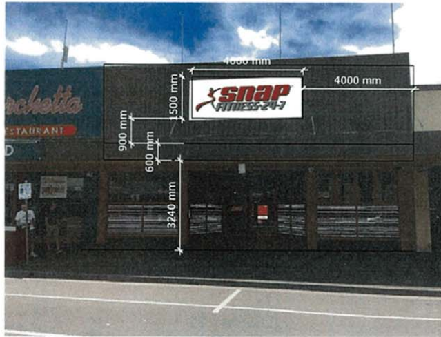
3D FABRICATED LOGO - FACADE illuminated LED modules
