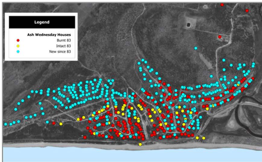
Figure 21 Dwellings in Fairhaven following Ash Wednesday fire
